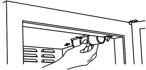
3. Replace the light bulb with an appliance bulb of the same wattage.
